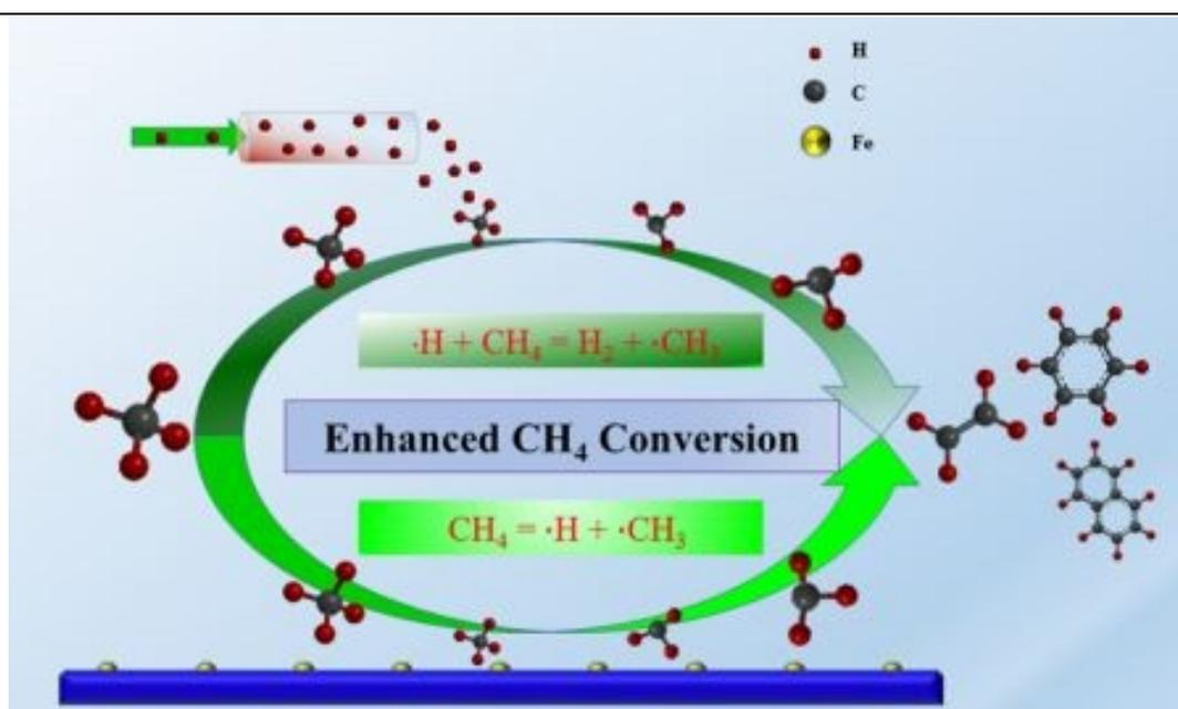
**Figure 5:** Single Fe sites in a silica matrix generate both methane and hydrogen radicals, which go through gas-phase C-C coupling to form ethylene (in addition to other useful products like aromatics and hydrogen). (Hao et al., 2019)
