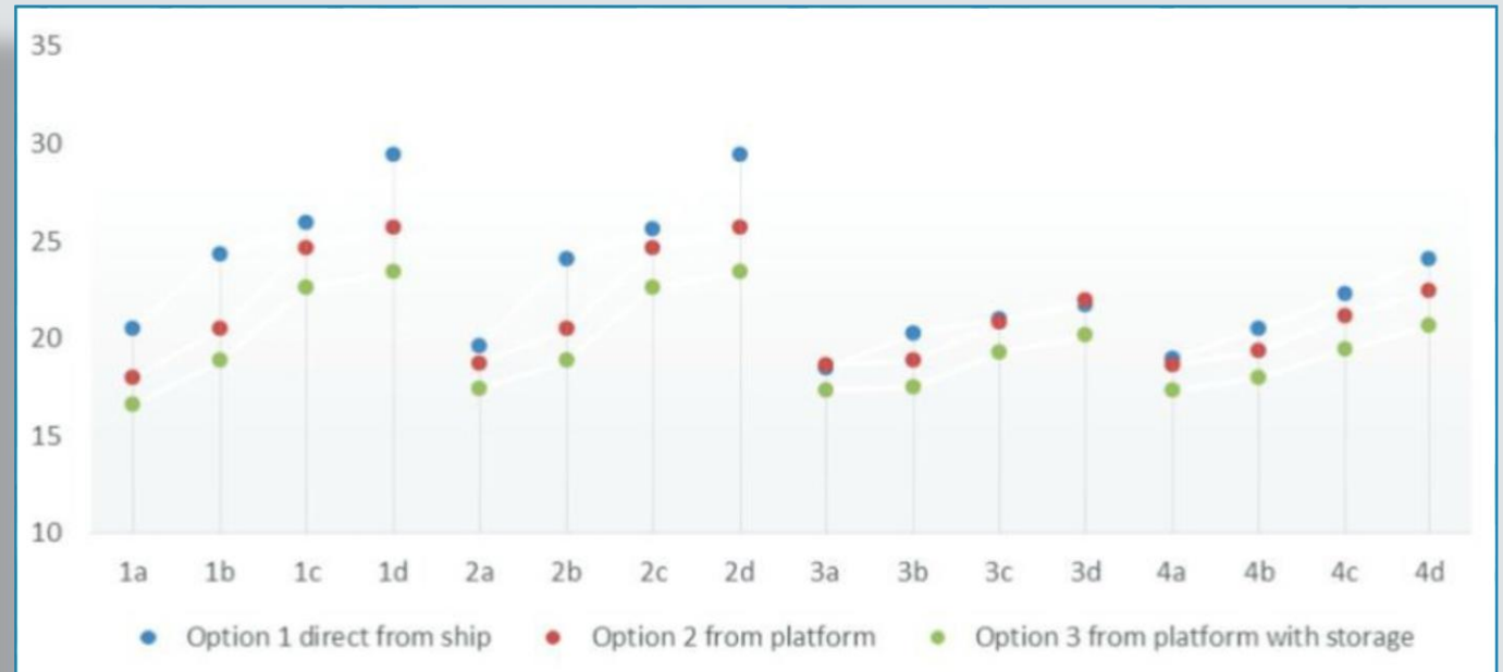
CO 2 Transportation Cost for the Different Reservoir Cases at a Shipping Distance of 800 Km
